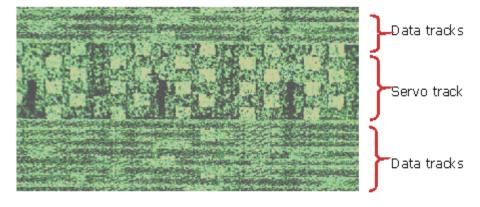
Figure 1. LTO Data Tracks and Servo Tracks
